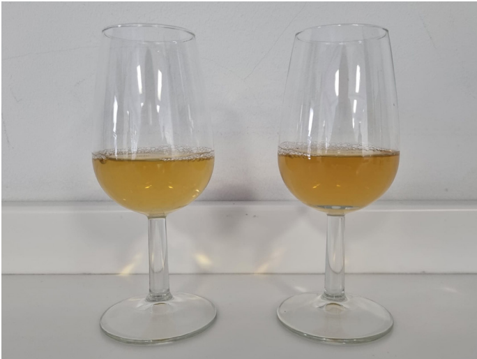
Fig. 1 Changes in colour by pasteurisation: fresh hot steep malt extract (left) and pasteurised hot steep malt extract (right)
