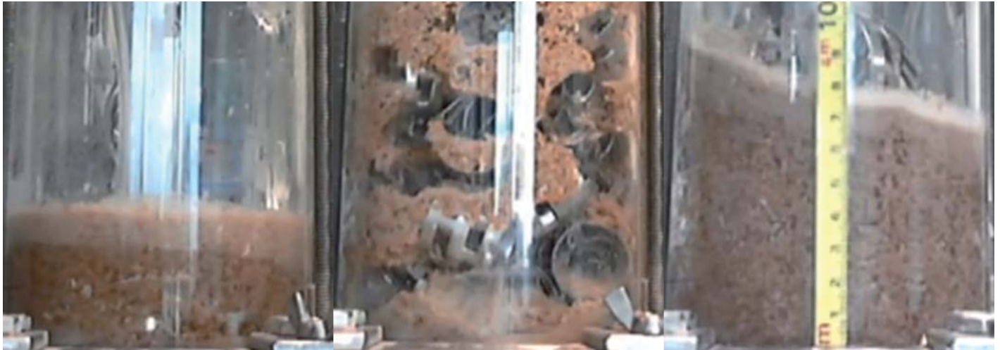
Fig. 7 Filter cakes after lautering (left to right) without and with Raflux rings and Top-Paks
