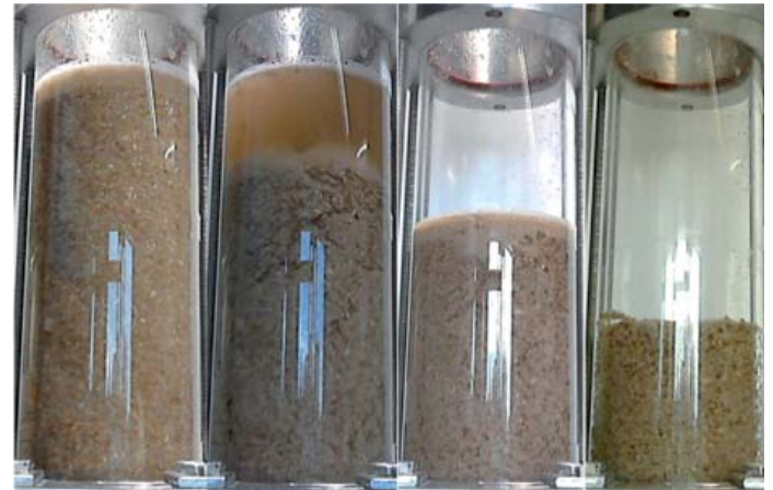
Fig. 5 Sub-stages of the lautering process identified during the reference procedure. From left to right: initial mash, sedimented cake, filtration and permeation, final cake compression.
