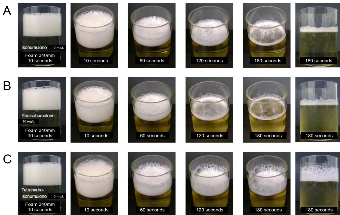
Fig. 7 Time-course photographs during foam collapse in FCT measuring glass: A, adding 10 mg/L of isohumulone; B, adding 10 mg/L of rho-isohumulone; C, adding 10 mg/L of tetrahydro-isohumulone
