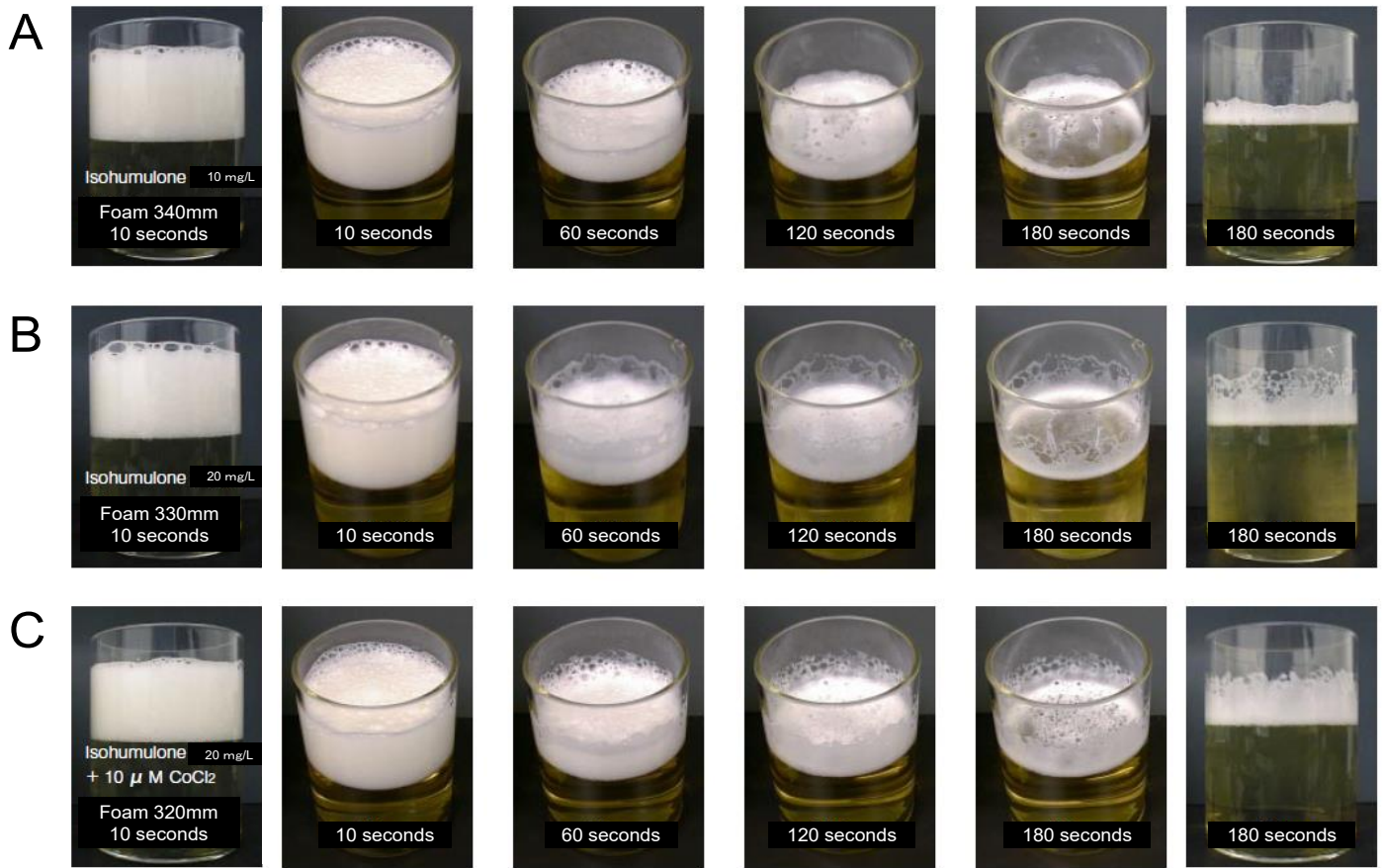
Fig. 5 Time-course photographs during foam collapse in FCT measuring glass: A, adding 10 mg/L of isohumulone; B, adding 20 mg/L of isohumulone; C, adding 20 mg/L of isohumulone and 10 μM CoCl 2
