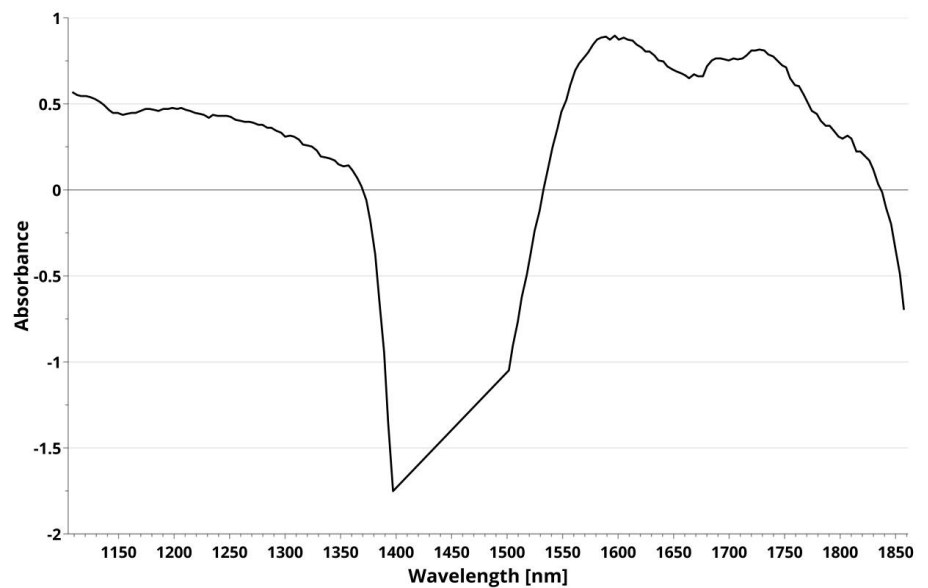
Fig. 4 Exemplary NIR spectrum at 90 \text{ }^\circ\text{C} and 10 L/h after wavelength selection and SNV
