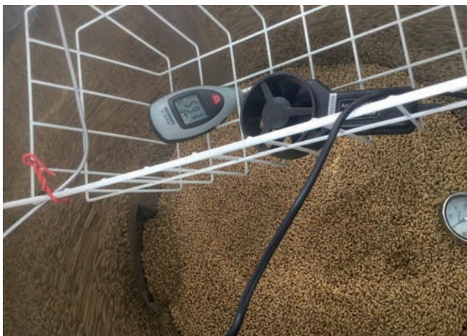
Fig. 10 Picture with Kilned Malt inside the Solar Kiln during the test
