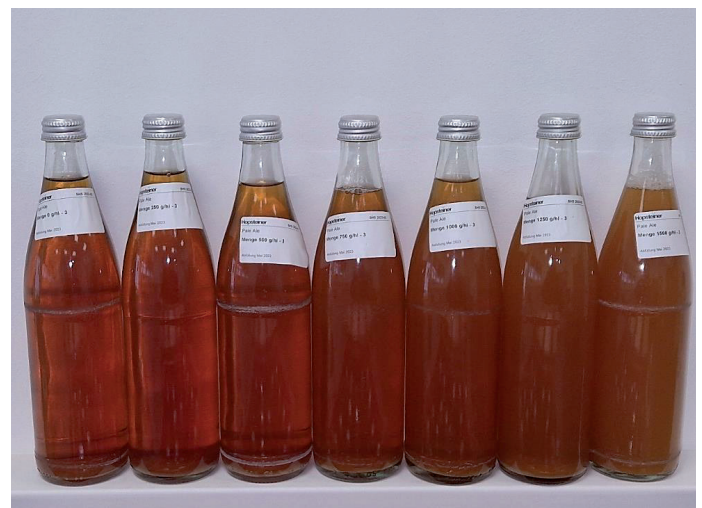
Fig. 5 TQ; visual appearance after 6 months of warm storage away from light; left to right: 0, 250, 500, 750, 1000, 1250, 1500 g pellets per hl
