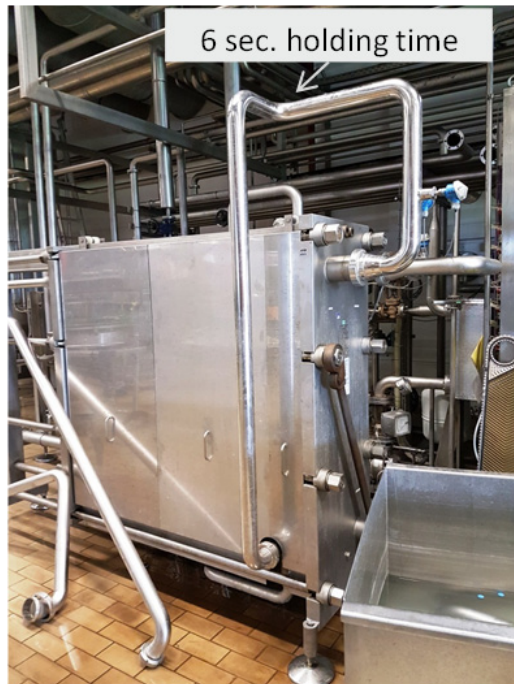
Fig. 2 Plate heat exchanger with a short heat-holding time of 6 seconds
