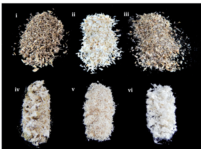
Fig. 6 Bleaching effect and the visible grade of released cellulose of active ECA chlorine on BSG and wheat straw. i: untreated spent grain; ii: BSG 120 h; iii: BSG DCT 0,5 h; iv: WS DCT 30 min; v: WS 6 h; vi: WS 120 h
