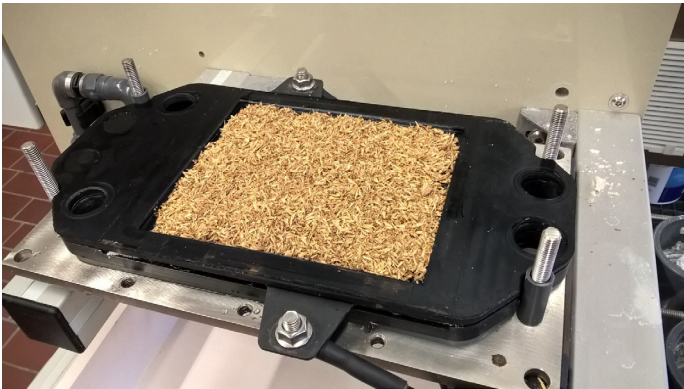
Fig. 2 Picture of the opened electrolysis cell filled with BSG before treatment. The cell is closed with the upper electrode
