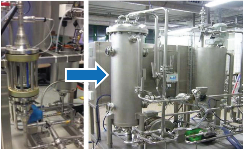
Fig. 2 Filtration cell (left), pilot filter with candles (right)
