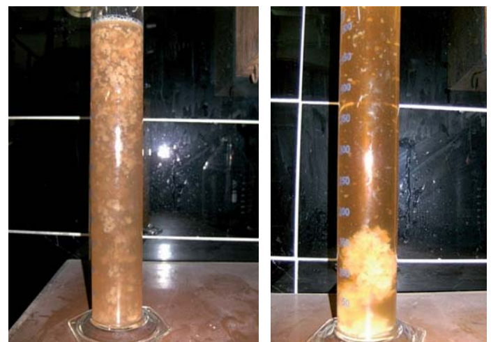
Fig. 4 Sedimentation of hot break materials in P7.2 and P7.1 experiments after 20 minutes rest; left, Beatrix variety; right, Irlbach variety
