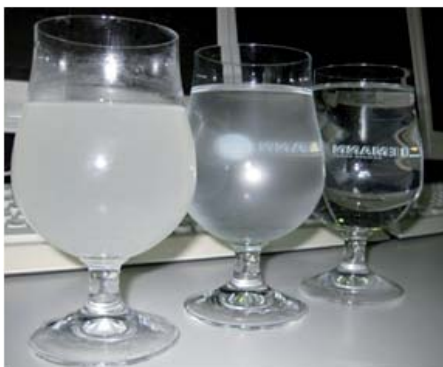
Fig. 5 Water samples from left to right – Feed sample, sample after the water switch and before the membrane, permeate sample after the membrane
