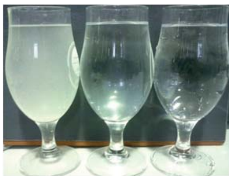
Fig. 6 Water samples from left to right – Feed sample, sample after activation of the water switch and before the membrane, permeate sample after filtration unit
