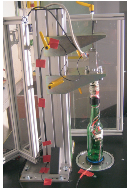
Fig. 3 Fixation of the bottle into the rotating equipment
