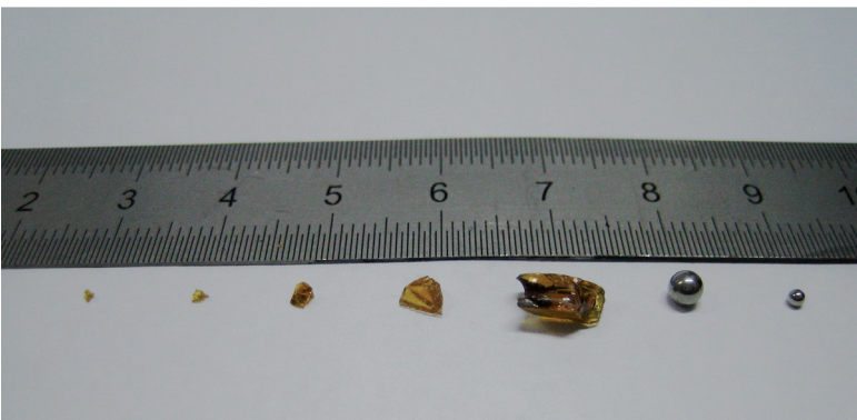
Fig. 5 Applied model particles: glass particles and steel spheres of different sizes
