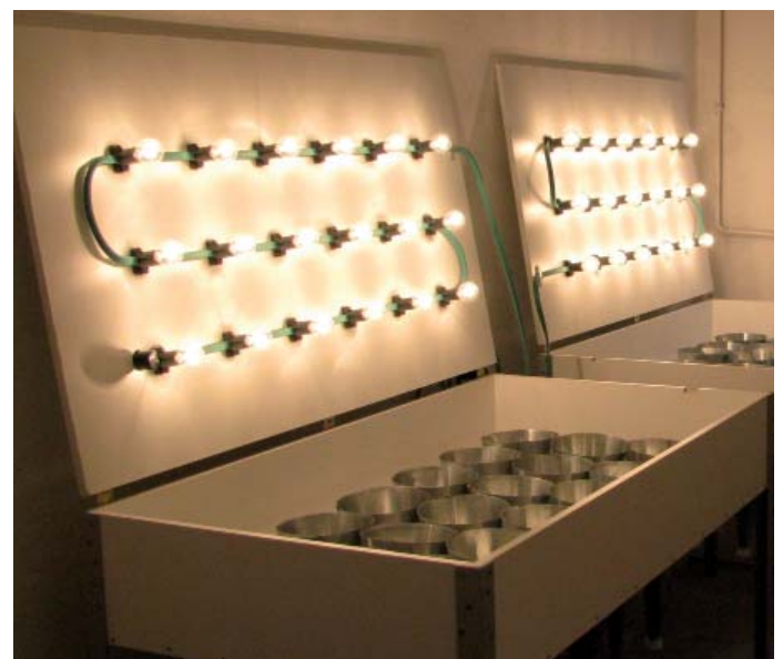
Fig. 1 Modified Berlese funnel device to expel arthropods by light and heat from green hop cones
