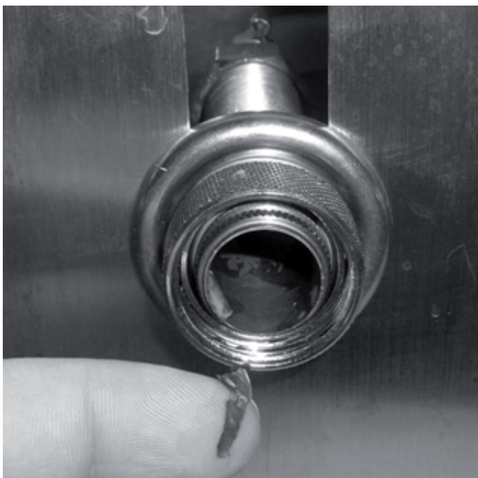
Fig. 10 Delamination of the internal nickel coating [15]
