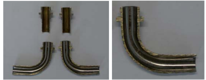
Fig. 6 Picture of a used hose nozzle sliced in half. The arrow refers to the areas where the coating is detached after the trials [14, 15]
