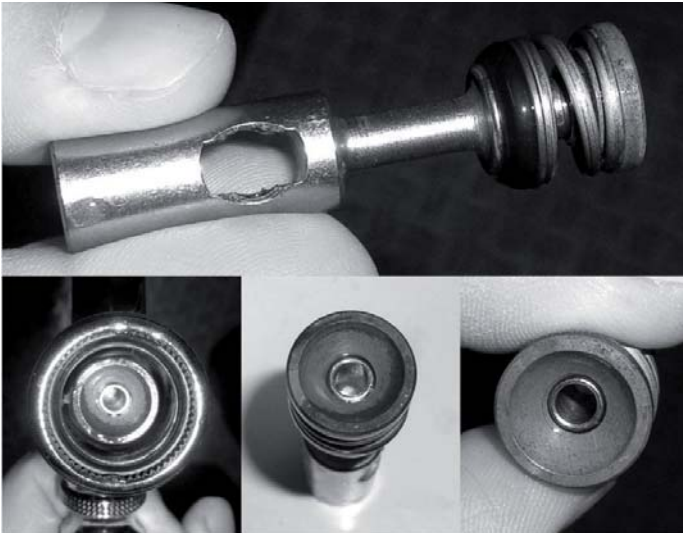
Fig. 11 Massive corrosion of the components
