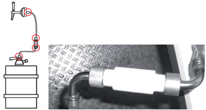
Fig. 1 Test setup for the hose nozzle testing. The circles show the places where the coated brass nozzles were used. On the right picture a double threaded piece is shown [14, 15]
