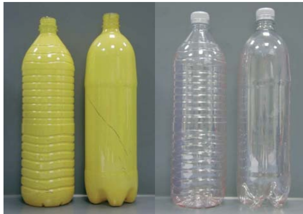
Fig. 6 Bottles with standard soiling substances: mustard (left) and Allura red AC® (right)
