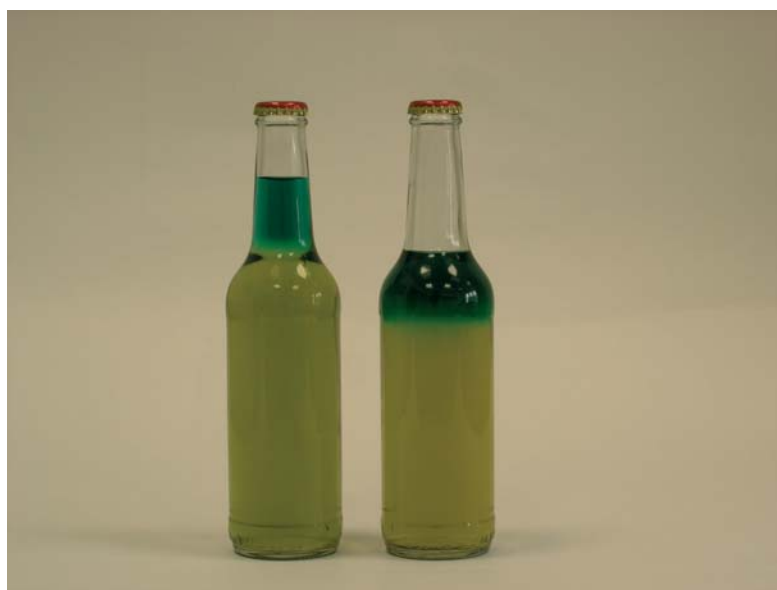
Fig. 3 Visualization of oxygen transfer from bottle neck to beer through reoxidation of the previously reduced form of methylene blue for two volumes of headspace loaded with air
