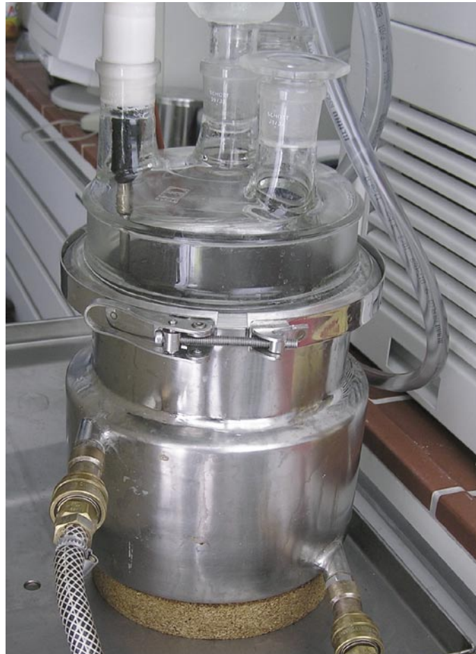
Fig. 1 Closed reactor with reflux condenser
