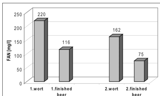
Fig. 1 FAN concentration in wort and finished beer in dependence on mashing-in temperature, 37°C (1.) and 63°C (2.)
