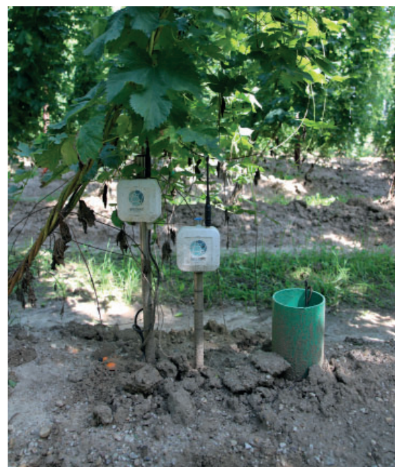
Fig. 4 Watermark and capacitive soil moisture sensors (Photograph by the author)
